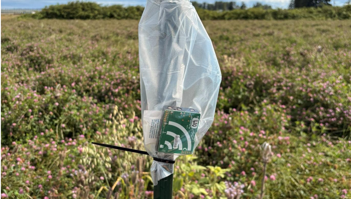
Photo 1 An ARU deployed in a pollinator mix grassland set aside.
